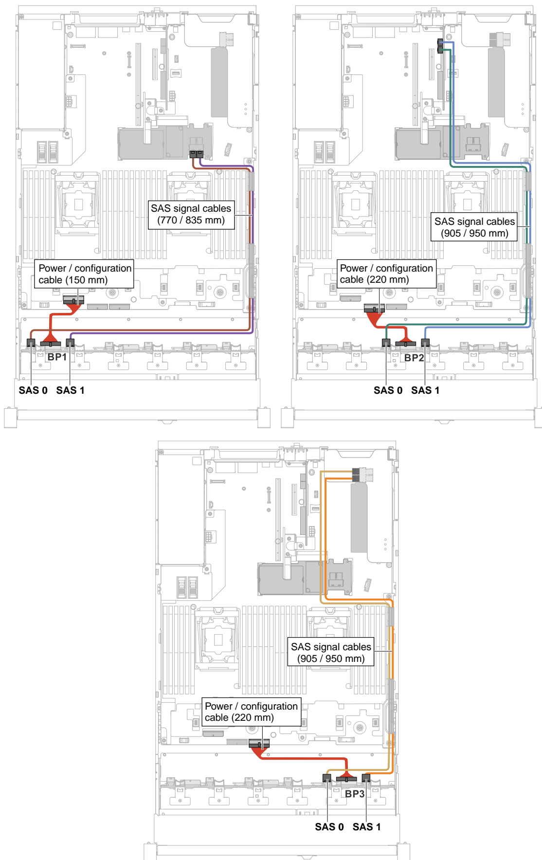
Figure 68. 24x2.5-inch hot-swap hard disk drive cabling
