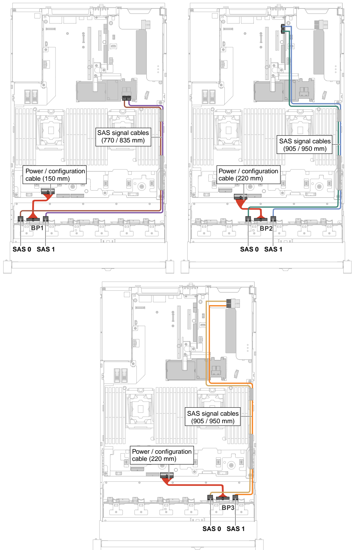
Figure 281. Cable routing
